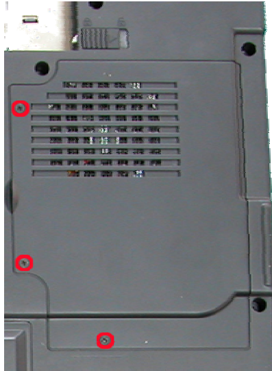
Fig. 10 Removing the screws retaining CPU cover
